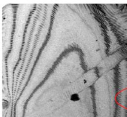
*Nano-drumming of graphite, visualized with 4D microscopy. (Nano Letters; image produced at Caltech)*
